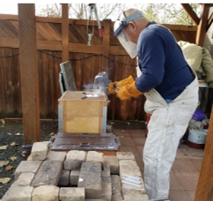
Pouring the molten metal into the sand mold. Time invested on a single cover is about 6 hours that includes clean up!
