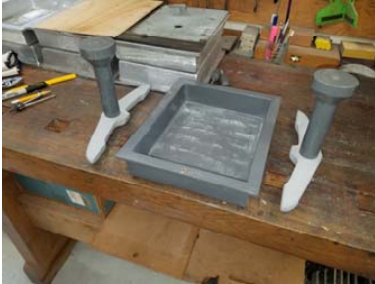
The pattern, runners and sprues ready for mold building.
