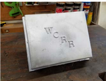
The sprues and runners have been trimmed up from the casting and are ready for finish machining.
