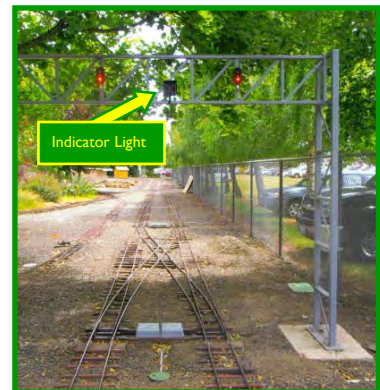
The "XOVER SELECT" switch must be held in the "||" or "X" position for three seconds to activate the electric switches. Both signals on the bridge go red until the switching process completes. This takes several seconds as each switch must turn individually in sequence.
