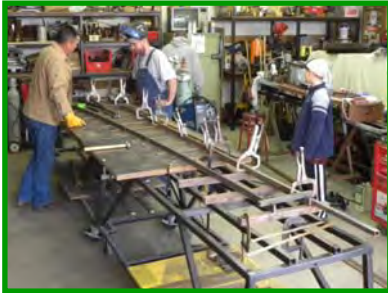
Vintage photo of turnout fabrication in Garry's Portland shop. (Trevor is much taller now.)
