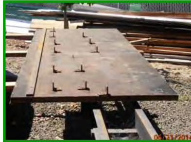
Old turnout template. It was constructed on thick particle board and was VERY heavy.
