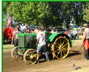
Trevor restarts the stalled tractor. The 1929 John Deere is started using the fly wheel. No electric start on this model! Scott said he developed "Popeye Biceps" doing this as a young lad.
