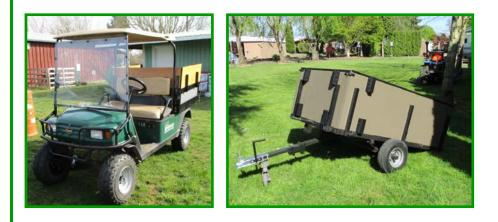
This winter Jeremy Johnson upgraded the EZGo with а new windshield. reinforced cab supports, tailgate and dump box extensions. He also upgraded the trailer with floor and side extensions with brackets for rake storage.
